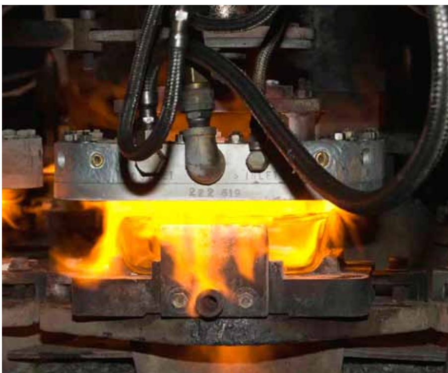
A Pyrex product passes underneath a fire polish burner which removes any sharp edges.
