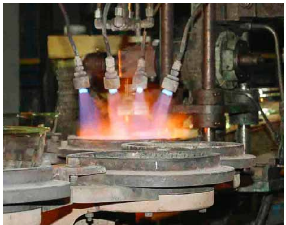
Energy intensive reheater burners keep process equipment hot to avoid inducing a temperature shock in the glassware.
