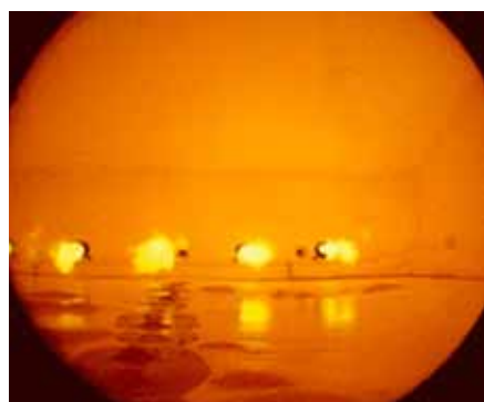
The glass furnace at World Kitchen uses gas oxygen burners and an electric boost to melt the raw glass to 1 400°C, seen here floating under the gas burners on the far side of the tank.
